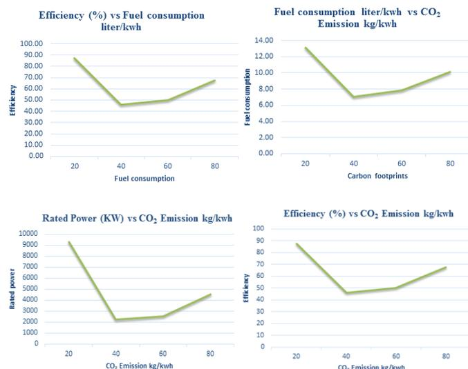
**Figure 2:** Relationship between Rated power, Fuel consumption, Carbon footprints, and Efficiency
