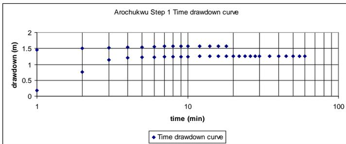
**Figure 9:** Time - drawdown curve of Arochukwu typical Lower Benue Trough shaley sandstone aquifer, Abia North.
