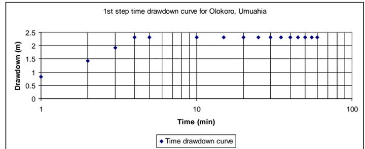
**Figure 12:** Time - drawdown curve of Olokoro-2, Umuahia typical NGB - Lower Benue Trough transitional boundary aquifer.
