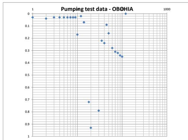
**Figure 5:** Time - drawdown curve of Obohia, typical Niger Delta basin aquifer in Abia south.
