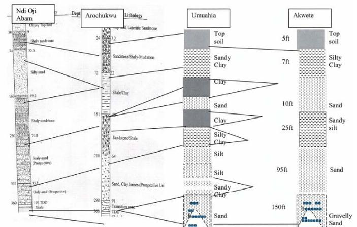
**Figure 14:** Aquifer geoelectric framework model correlation across the Lower Benue Trough, transitional boundary and Niger Delta basins.
