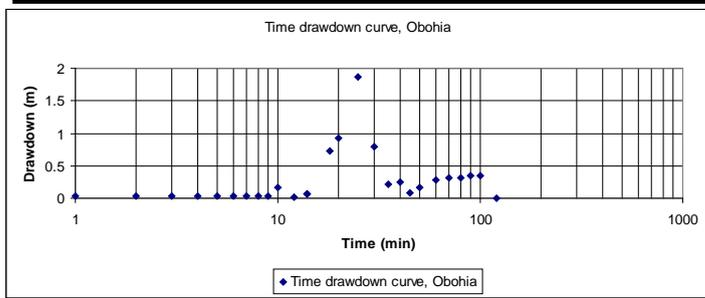
**Figure 6:** Time - drawdown curve of Obohia-2, typical Niger Delta basin aquifer in Abia south.
