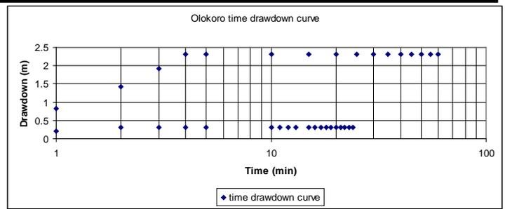
**Figure 11:** Time - drawdown curve of Olokoro, Umuahia typical NGB - Lower Benue Trough transitional boundary aquifer.
