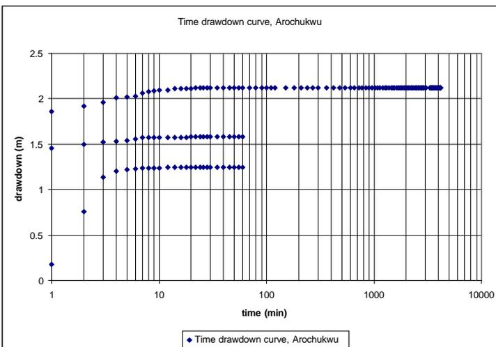
**Figure 10:** Time - drawdown curve of Arochukwu-2 typical Lower Benue Trough shaley sandstone aquifer, Abia North.
