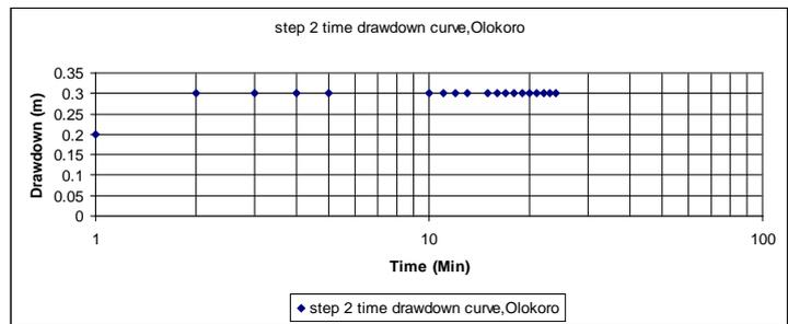
**Figure 13:** Time - drawdown curve of Olokoro-3, Umuahia typical NGB - Lower Benue Trough transitional boundary aquifer.
