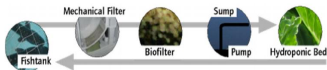
Figure 2: Basic aquaponics system layout
